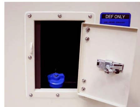
Lockable external DEF fill
